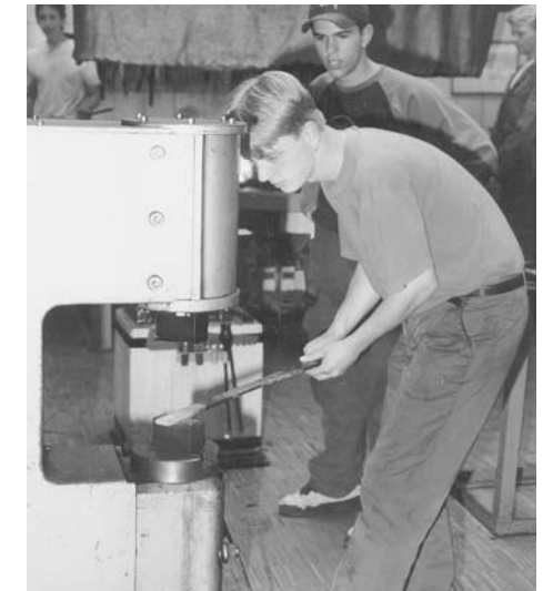
Fine forging with the air hammer.
