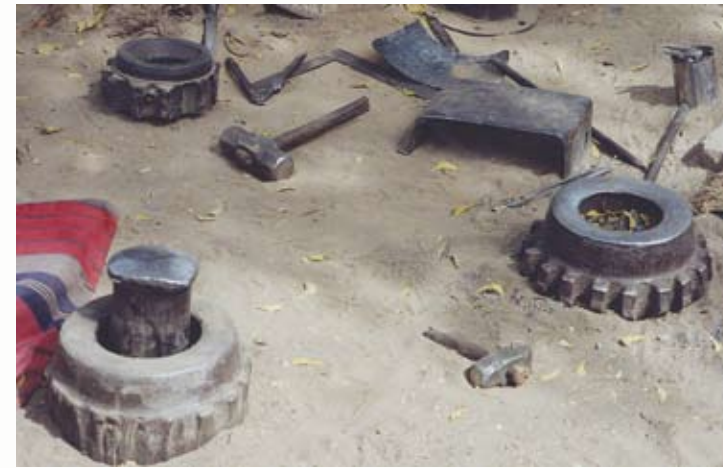
The shop setup, for sinking and raising vessels. Very large truck bearings are utilized for sinking forms.
