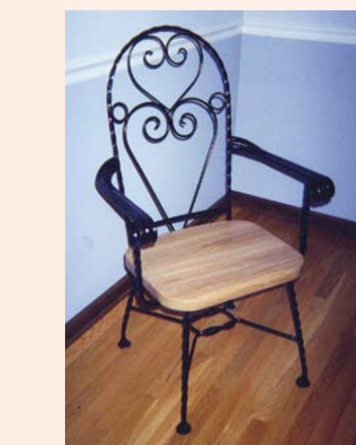
Edward Eichholz, Wilmington, Delaware Back of chair is 1/2" solid square bar, twisted. The small rings are 1/4" square twisted. The hearts are 5/16" round stock. Arms are railing top cap. Arm supports and legs are 1/2" solid square, legs were split in quarters and splayed to fit the feet. Seat is white oak hand-worked by this blacksmith.
