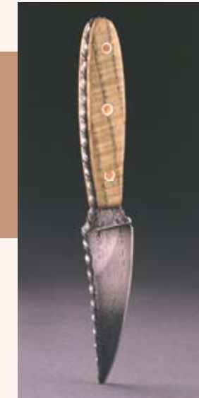
BUGS knife. 5 3/4" x 3/4" x 3/8". 15N20, 1084, ash, copper, silver
