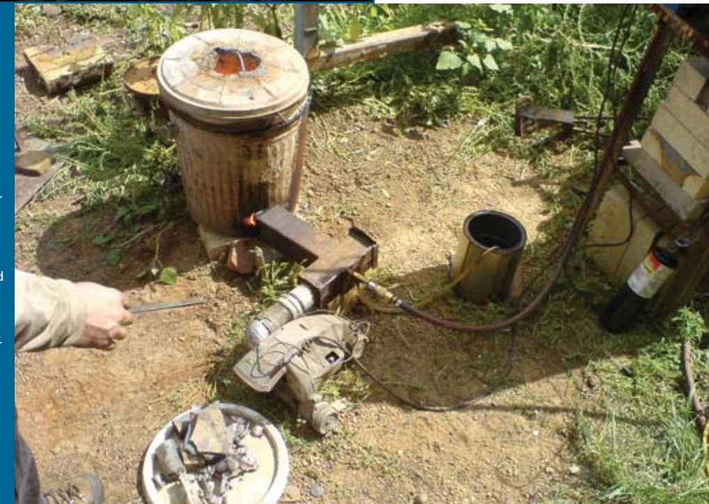
Melting bronze for a casting. The fuel is in the golden can, an old vacuum cleaner serves as air blower.
