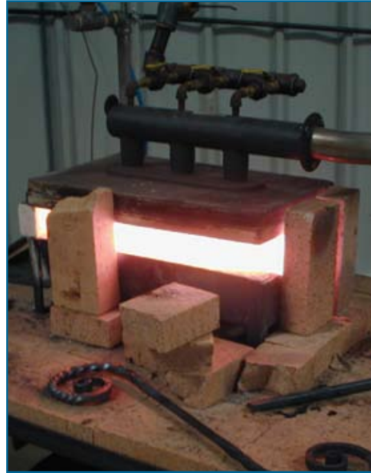
After many adjustments to the Mankel Knifemaker forge, the system ran on gas captured from the closed landfill. Note the intensity of the flame, indicating that the system has reached forging temperature.
