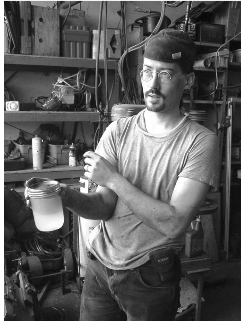
Washing out the soap from a sample of biodiesel.
