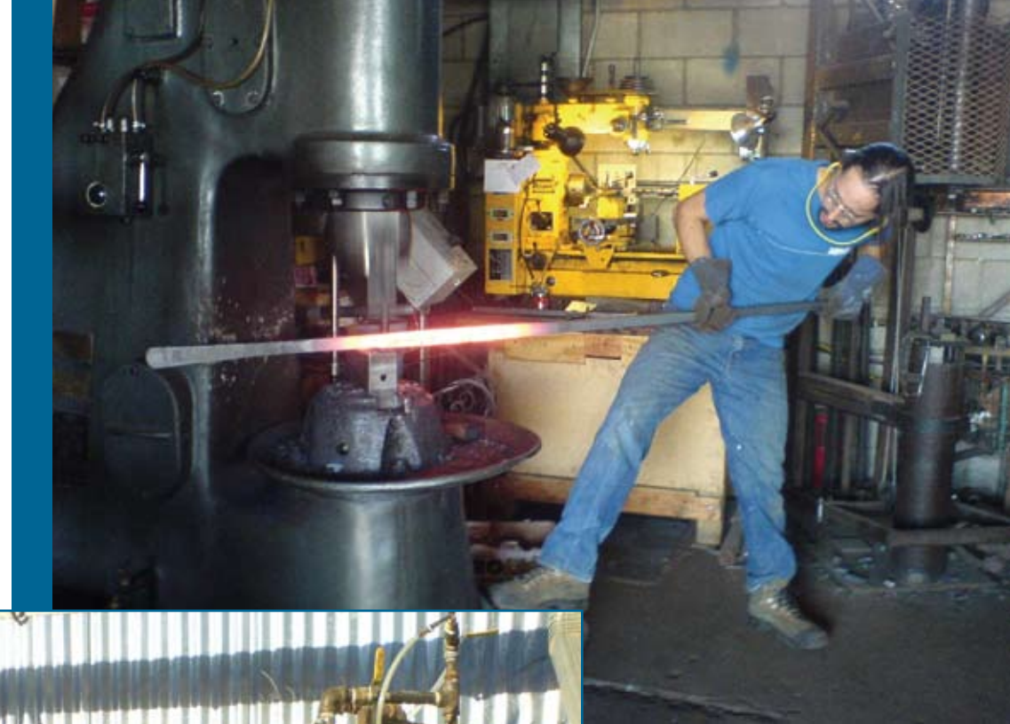
Forging the heated iron bar under the power hammer.
