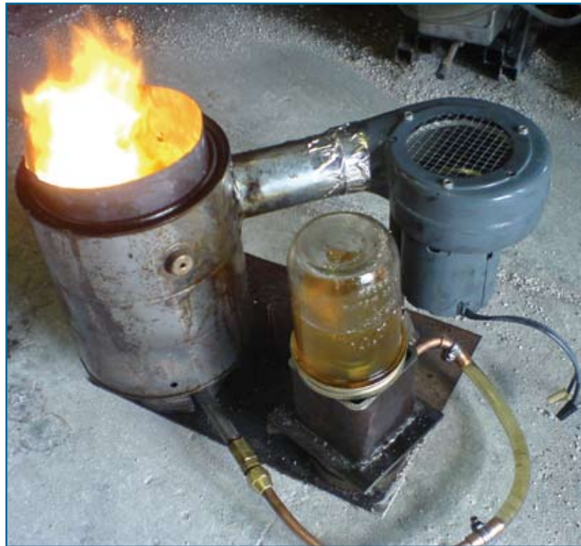
An experimental vegetable oil burner, one of many Cameron built.
