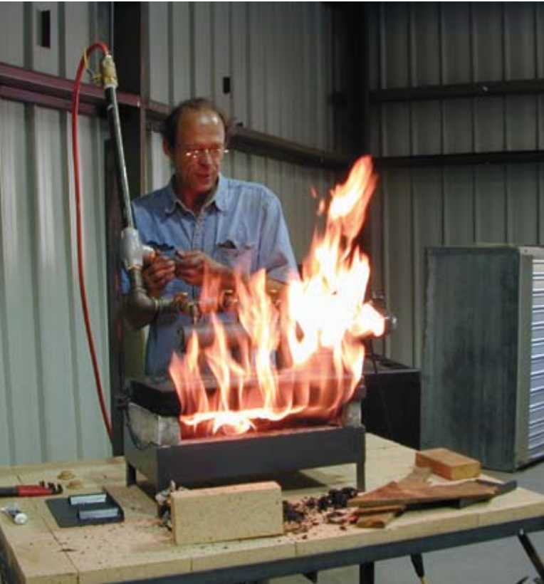
William Rogers adjusting a reducing flame that seeks oxygen and climbs out of the firebox.
