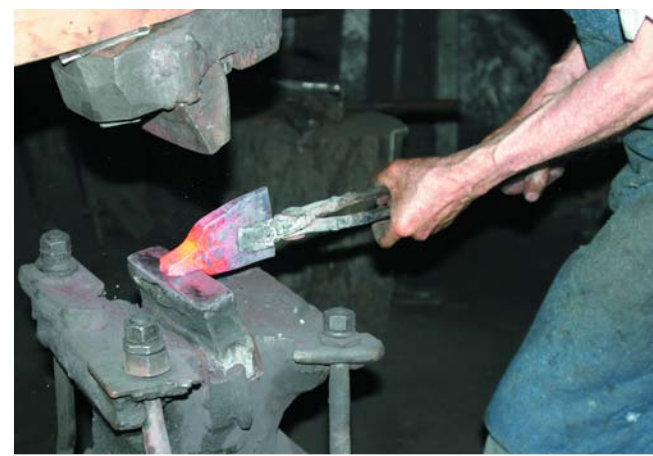
Forging the shoulder under the power hammer.
