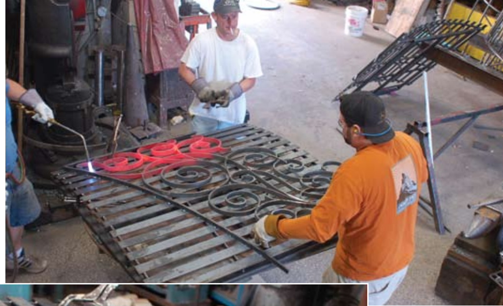
Shop photos showing fabricated forms, on which we bend decorative panels. Each radiused form is fabricated based on the required centerline radius of the on-site stairway. The panel is heated in a Johnson gas forge and clamped in position on the form and tweaked with a rosebud torch into final form. Note the bridge welded to the form to maintain proper slope of the panel.
