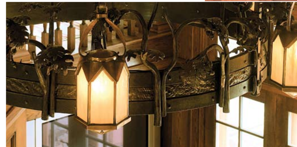
"Victoria Woods" chandelier. For private residence. Forged mild steel. Glasswork by Mark Read. Mild steel frame, bronze lanterns. 7'4" tall with 10' hanger. 6' diameter bottom tier, 4' diameter top tier. Linseed/wax finish.
