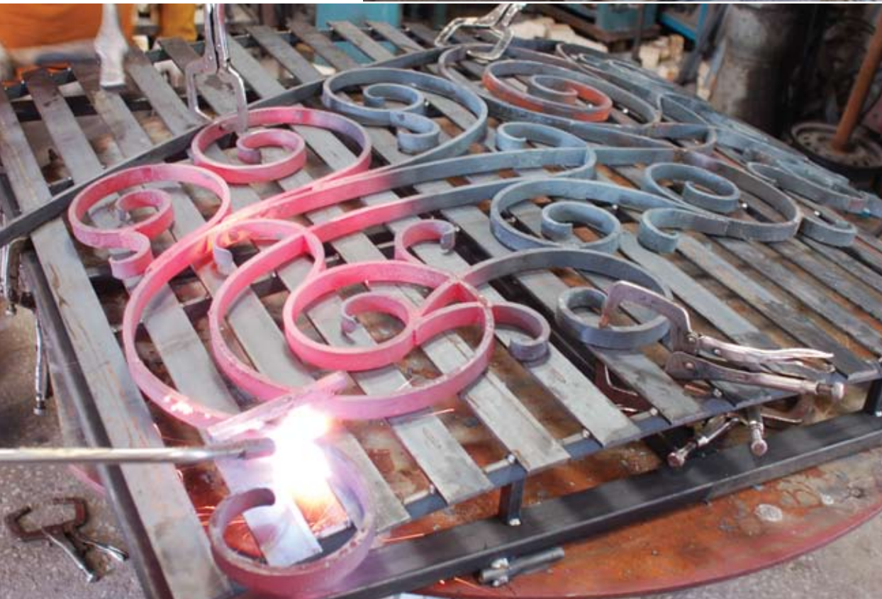
Shop photos showing fabricated forms, on which we bend decorative panels. Each radiused form is fabricated based on the required centerline radius of the on-site stairway. The panel is heated in a Johnson gas forge and clamped in position on the form and tweaked with a rosebud torch into final form. Note the bridge welded to the form to maintain proper slope of the panel.
